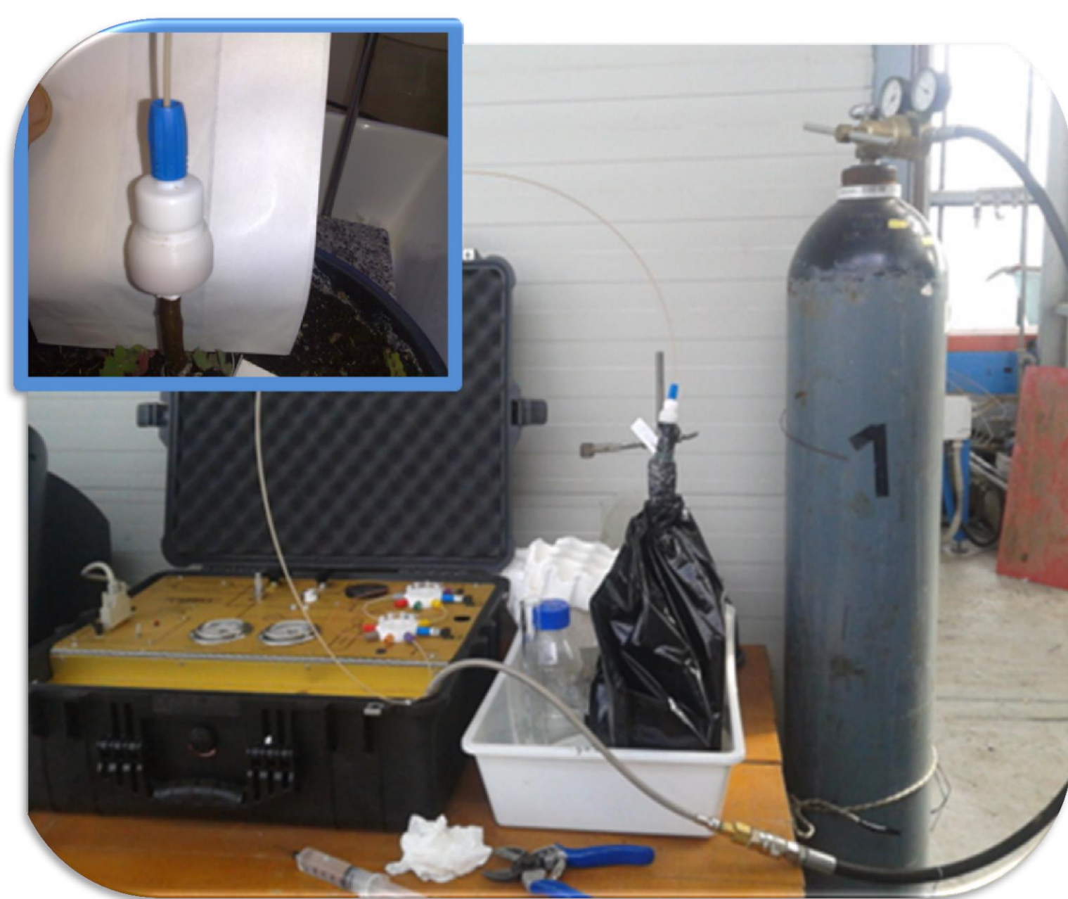
A view of the HCFM. In the inset: the coupling hedge fitted to a cut trunk
